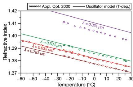
Fig. 5 RI measurements at four different wavelengths for an aqueous solution containing  $\text{H}_2\text{SO}_4$  and  $\text{HNO}_3$  ( $\phi_{\text{H}_2\text{SO}_4} = 0.1741$  and  $\phi_{\text{HNO}_3} = 0.1741$ ) from ref. 32 compared to the temperature-dependent effective oscillator model ( $\kappa = -0.0015 \text{ K}^{-1}$ ).
