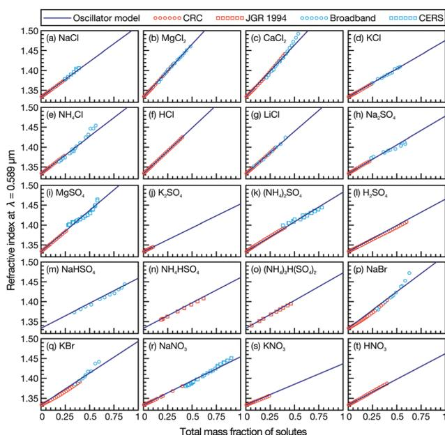
**Fig. 1** Comparison between bulk refractometer measurements (red points), single particle measurements (blue points), and effective oscillator calculation (solid line) for various aqueous inorganic solutions as a function of mass fraction of solute. All RI measurements are at  $\lambda = 0.589\ \mu\text{m}$ . Bulk measurements are from either ref. 11 (labeled 'CRC') or ref. 12 (labeled 'JGR 1994').
