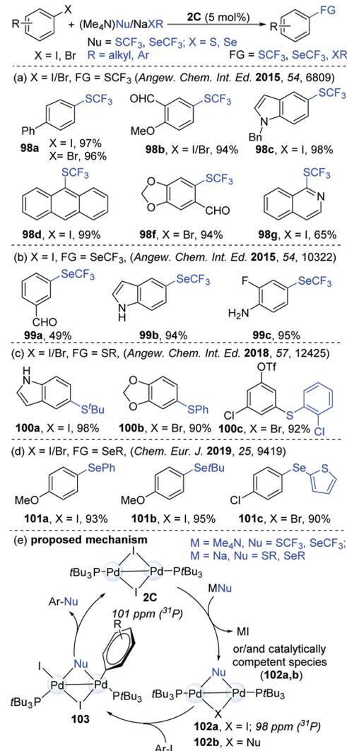
Scheme 26 The efficient organic transformation of aromatic halides catalyzed by  $\text{Pd}(\text{I})$  dimer.
