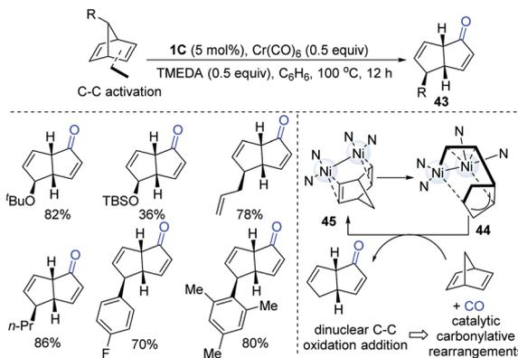
**Scheme 11** Dinuclear Ni-catalyzed carbonylative rearrangement of 7-substituted norbornadiene.
