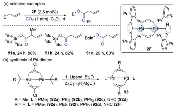
Scheme 23 Carboxylation of different allyls with CO<sub>2</sub> catalyzed by Pd-dimer.
