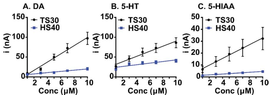
Fig. 3 Sensitivity comparison for TS30 and HS40 fibers. All calibration curves were conducted from 1 μM to 10 μM. (A) Dopamine (waveform:  $-0.4$  V to  $1.3$  V,  $400$  V s $^{-1}$ ,  $n = 6-10$ ), (B) 5-HT, and (C) 5-HIAA (waveform for TS30:  $0.2$  V to  $1.0$  V, down to  $-0.1$  V and back to  $0.2$  V,  $1000$  V s $^{-1}$ ; HS40:  $-0.4$  V to  $1.3$  V,  $400$  V s $^{-1}$ ,  $n = 8-10$ ).
