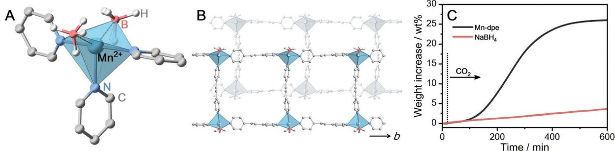
Fig. 3 (A) Local coordination geometry of **Mn-dpe**. (B) Packing structure of the extended 1D ladders of **Mn-dpe**. (C) Isothermal TGA profiles of **Mn-dpe** and  $\text{NaBH}_4$  under  $\text{CO}_2$  flow (0.1 MPa, 30  $\text{mL min}^{-1}$ ) at 40 °C.
