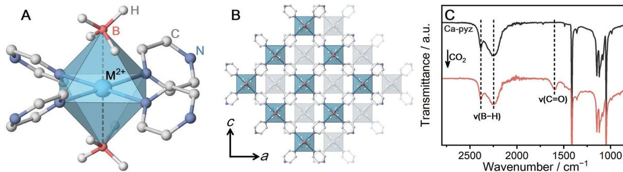
Fig. 1 (A) Local coordination geometry of  $M$ -pyz ( $M = \text{Mg}^{2+}, \text{Ca}^{2+}, \text{Mn}^{2+}$ ). (B) ABAB stacking structure of the extended 2D layers of  $M$ -pyz ( $M = \text{Mg}^{2+}, \text{Ca}^{2+}, \text{Mn}^{2+}$ ). (C) IR spectra of  $\text{Ca-pyz}$  before and after  $\text{CO}_2$  adsorption at  $25^\circ\text{C}$ .
