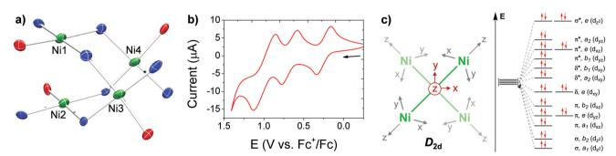
Fig. 1 (a) Partial solid-state structure of [Ni4] highlighting the inner core (see Fig. S15 for full structure, ESI†). (b) CV of [Ni4] in TCE (1 mM of [Ni4], 0.1 M [Bu<sub>4</sub>N][PF<sub>6</sub>] supporting electrolyte), glassy carbon working electrode, Pt wire counter electrode, and Ag wire pseudo-reference electrode. (c) Partial d-orbital splitting diagram for a  $D_{2d}$  tetrametallic core, ignoring ligand  $\pi$  interactions.
