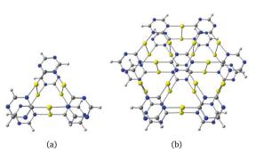
Fig. 7 Double-decker dimer structures of gold-containing  $\gamma$ -graphyne fragments belonging to the  $D_3$  and  $D_{3d}$  point groups. The HOMO-LUMO gaps at the B3LYP level are 3.55 eV and 2.68 eV for (a) and (b), respectively.
