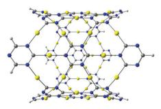
Fig. 8 Gold-nanotube complex constructed by using a fragment of a carbon nanotube of  $\gamma$ -graphyne. The molecular structure belongs to the  $C_{4v}$  point group and has a large HOMO-LUMO gap of 2.90 eV at the B3LYP level.
