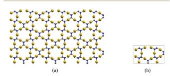
Fig. 4 The gold-containing two-dimensional structure analogous to (a) β-graphyne and (b) its unit cell.
