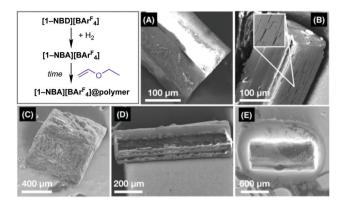
Fig. 2 SEM images of different single-crystal samples in polymer graftingfrom experiments. (A) [1-NBD][BAr $^{F}_{4}$ ]. (B) [1-NBD][BAr $^{F}_{4}$ ] + H<sub>2</sub> to form [1-NBA][BArF<sub>4</sub>]. Inset shows microcracks. (C) [1-NBA][BArF<sub>4</sub>]@poly-(ethylvinylether) formed after exposure to EVE for 30 seconds, (D) 2.5 minutes EVE exposure. (E) 15 minutes EVE exposure.
