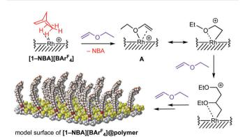
**Fig. 4** Suggested mechanism of grafting-from cationic surface polymerisation to form **[1-NBA][BAr** $^{F}_{4}$ **]@poly(ethylvinylether)**. [BAr $^{F}_{4}$ ] $^{-}$  anions not drawn.
