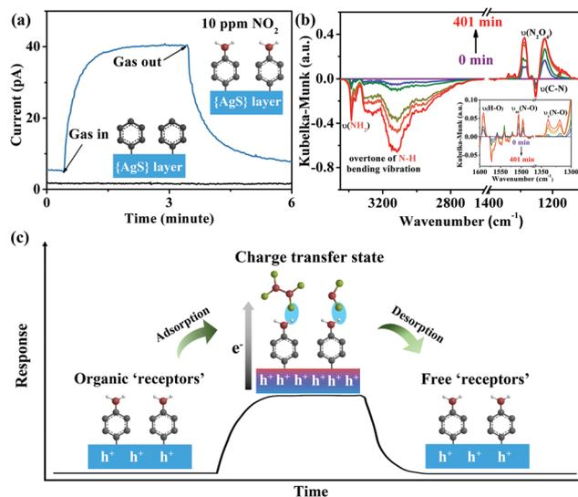
**Fig. 4** (a) Response–recovery curves of Ag(SPh-NH<sub>2</sub>) (blue) and Ag(SPh) (black) to 10 ppm NO<sub>2</sub>. (b) *In situ* DRIFT Spectra for Ag(SPh-NH<sub>2</sub>) exposed to NO<sub>2</sub> as a function of time. (c) Possible NO<sub>2</sub> sensing mechanism for Ag(SPh-NH<sub>2</sub>).
