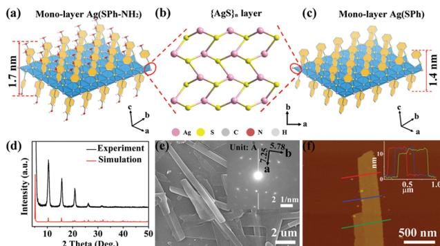
**Fig. 1** (a and c) Mono-layer structures of Ag(SPh-NH<sub>2</sub>) and Ag(SPh). (b) 2D {AgS}<sub>n</sub> layer of Ag(SPh-NH<sub>2</sub>) and Ag(SPh). Hydrogen atoms of the benzene ring have been omitted for clarity. (d) Experimental and simulated PXRD patterns of Ag(SPh-NH<sub>2</sub>). (e) SEM image of few-layer Ag(SPh-NH<sub>2</sub>), inset is its selected area electron diffraction pattern. (f) Typical AFM image of few-layer Ag(SPh-NH<sub>2</sub>).
