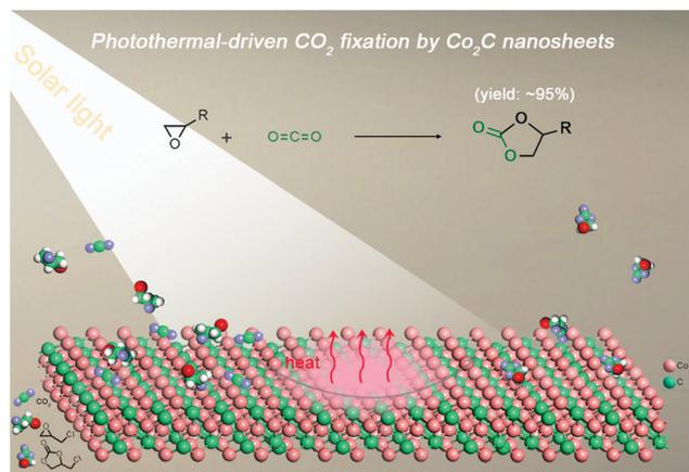
**Scheme 1** Illustration of the photothermal-driven cycloaddition of CO<sub>2</sub> with epoxides catalyzed by Co<sub>2</sub>C nanosheets of the nanoflower.
