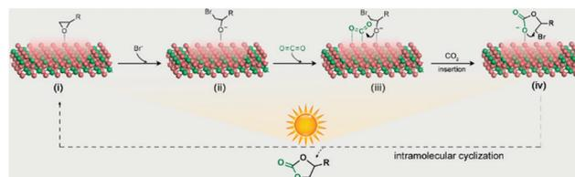
**Fig. 3** The proposed mechanism of  $\text{Co}_2\text{C}$  catalysed  $\text{CO}_2$  cycloaddition with epoxides under light irradiation.
