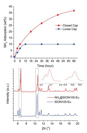
Fig. 2 (top) NH<sub>3</sub> adsorption curve for **SION105-Eu** as a function of time: (bottom) PXRD pattern of the SION105-Eu sample after 6 hour of NH<sub>3</sub> vapour adsorption in comparison to the as-made sample. Inset: The appearance of new peaks within the selected regions.
