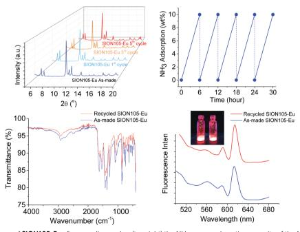
Fig. 3 (top left) PXRD patterns of SION105-Eu after recycling cycles; (top right) the NH<sub>2</sub> vapour adsorption capacity of the MOF remains the same after 5 cycles; (bottom) FTIR spectra and luminescence emission ( $\lambda_{ex}$  = 360 nm) of the as-made and recycled **SION105-Eu**. The inset shows the red emission under UV radiation of the as-made (left) and recycled (right) materials
