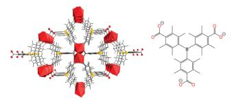
Fig. 1 (left) Structure of SION105-Eu, with Eu ions shown as red polyhedra and H atoms omitted for clarity; (right) ligand tctb<sup>3-</sup>
