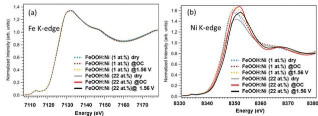
**Fig. 2** (a) Fe and (b) Ni XANES spectra of 1% Ni ( $\beta$ -FeOOH:Ni) and 22% Ni ( $\beta$ -FeOOH:Ni surface-decorated with  $\text{Ni}(\text{OH})_2$ ) acquired under dry, OC potential and OER potential (+1.56 V) conditions.
