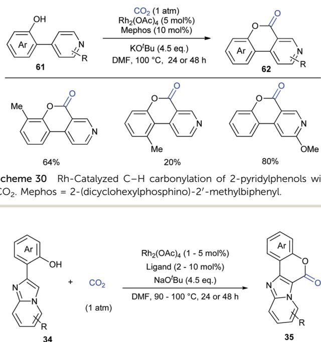
**Scheme 30** Rh-Catalyzed C–H carbonylation of 2-pyridylphenols with CO<sub>2</sub>. Mephos = 2-(dicyclohexylphosphino)-2'-methylbiphenyl.
