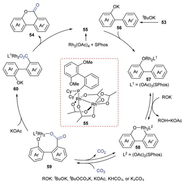
**Scheme 29** The catalytic cycle of Rh-catalyzed lactonization reaction.
