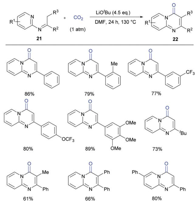
Scheme 13 Transition metal-free carbonylation of C(sp<sup>3</sup>)-H bonds in pyridylamines with CO<sub>2</sub> in the presence of LiO<sup>t</sup>Bu.
