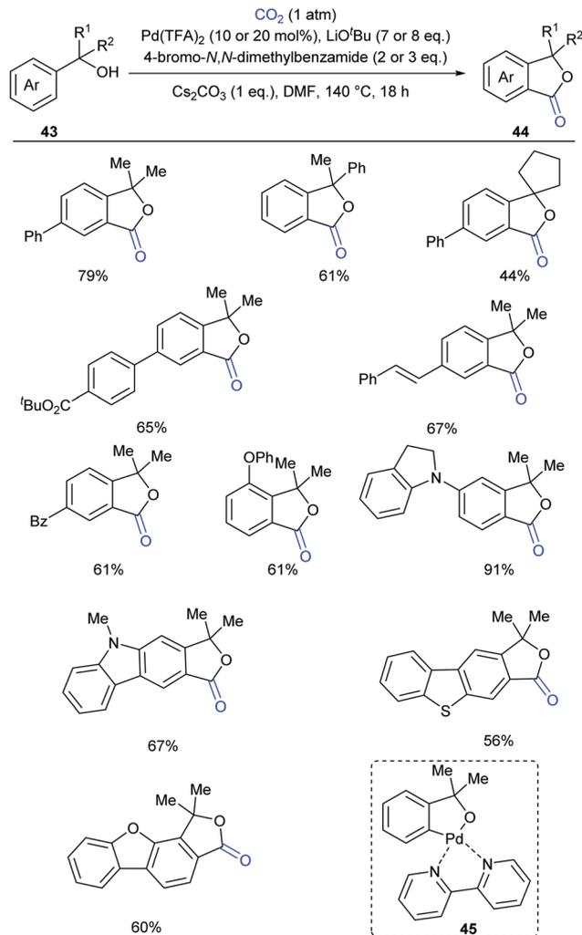
**Scheme 26** Pd-Catalyzed carbonylation of tertiary benzylic alcohols with CO<sub>2</sub>.
