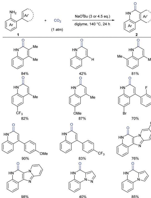
Scheme 3 Transition metal-free carbonylation of C(sp<sup>2</sup>)–H bonds in *o*-alkenyl- and *o*-heteroaryl-anilines with CO<sub>2</sub> in the presence of NaO<sup>t</sup>Bu.
