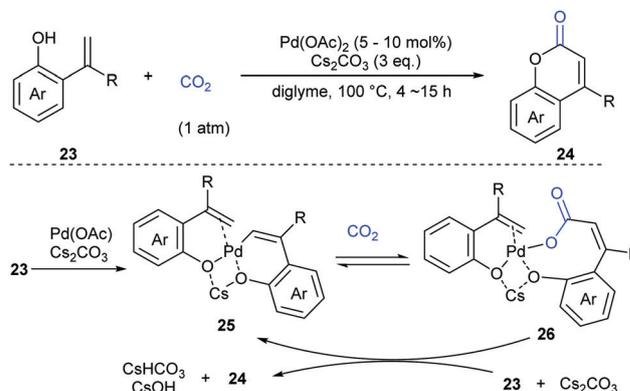
**Scheme 17** Proposed mechanism for Pd-catalyzed carbonylation reaction.
