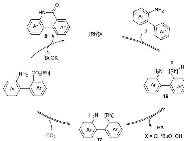
Scheme 10 The catalytic cycle of Rh(I)-catalyzed lactamization.
