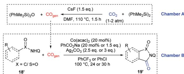
Scheme 11 Transition-metal-catalyzed carbonylation of benzamides with CO<sub>2</sub>.
