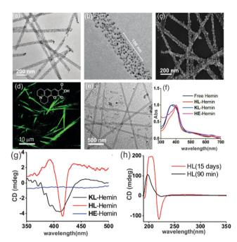
Fig. 2 (a) TEM image of negative-AuNPs bound with HL and (b) an enlarged TEM image of a negative-AuNP bound with HL. (c) SEM image of AuNP-HL nanotubes. (d) CLSM image ( $\lambda_{\rm ex}$  = 488 nm) of Coumarin 343 dye bound to HL. (e) TEM image of hemin-HL. (f) Normalized UV-Vis spectra of free hemin, and hemin in the presence of HL, KL, and HE at pH 3. (g) CD spectra of hemin bound HL, KL, and HE. (h) CD spectra of HFIP treated HL after 90 min and 15 days.
