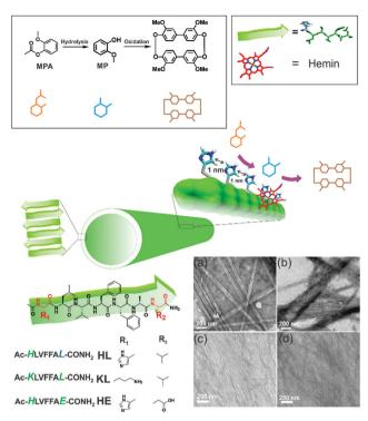
**Fig. 1** Scheme showing cascade reaction on nanotube surface, and chemical structures of amyloid, MPA, MP and the oxidation product. TEM and SEM images of self-assembled **HL** (a and c) and **KL** (b and d) respectively.
