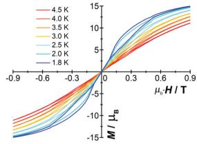
Fig. 2 Magnetic hysteresis of  $[Cp*Dy]_6$  at indicated temperatures with a sweep rate of 0.002 T s<sup>-1</sup>.
