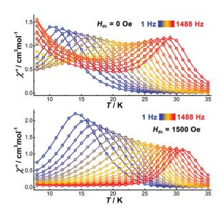
Fig. 3 Temperature dependence of the out-of-phase part of the ac susceptibility for [Dy-Cp\*]<sub>6</sub> under zero (top) and 1500 Oe dc field (bottom).
