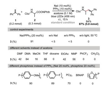
Scheme 1 Key reaction parameters. Reaction conditions: 1 (0.2 mmol, 1.0 eq.), 2 (0.3 mmol, 1.5 eq.), Nal (10 mol%), PPh3 (10 mol%), acetone (2.0 mL), irradiation with blue LEDs (456 nm) at room temperature for 15 h under an argon atmosphere. Yield of the isolated product.
