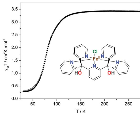
Fig. 1 Magnetic properties of  $[\text{Fe}^{\text{II}}(\text{Py5OH})\text{Cl}](\text{PF}_6)$  powder in the form of  $\chi_{\text{M}}T$  vs.  $T$  recorded in cooling (open circles) and warming (filled circles) modes with a scan rate of  $2 \text{ K min}^{-1}$ . The molecular structure of the complex is shown as an inset.
