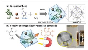
Fig. 1 Schematic of the (a) one-pot synthesis of the HRP/MNP@ZIF-8 composite, and (b) its usage as catalyst for the H<sub>2</sub>O<sub>2</sub>-mediated oxidation of pyrogallol to purpurogallin, with the possibility of magnetic collection.
