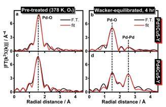
**Fig. 3**  $k^3$ -Weighted Fourier transform magnitude (non-phase shift corrected) of the Pd K-edge EXAFS spectra of (a and b) Pd1Cu5-Y and (c and d) Pd4Cu5-Y in different reaction conditions (FT performed in the 3–11 Å $^{-1}$  range and fitted in R space in the 1–3 Å range; black: magnitude of FT, red: best fit). The corresponding  $k^3$ -weighted Pd K-edge EXAFS spectra are shown in Fig. S8, ESI. $^{\dagger}$
