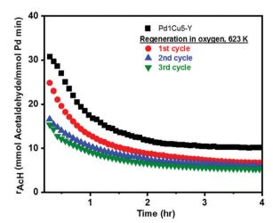
Fig. 4 Ethylene oxidation over Pd1Cu5–Y and the regenerated catalyst (3 subsequent reactivation cycles) under standard Wacker conditions vs. time-on-stream (TOS). Wacker conditions: 378 K, 0.86 kg<sub>cat</sub> s mol<sup>-1</sup>. Gas feed consists of  $C_2H_4$ :  $H_2O$ :  $O_2$  at a 1:7:10 molar ratio.
