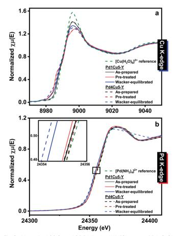
**Fig. 2** Normalized (a) Cu and (b) Pd K-edge XANES spectra of Pd-Cu/Y. Wacker conditions: 378 K,  $0.86~kg_{cat}~s~mol^{-1}$ . Gas feed consists of  $C_2H_4$ :  $H_2O:O_2$  at a 1:7:10 molar ratio. Inset: Magnification of (b) Pd K-edge XANES spectra at half-edge height.
