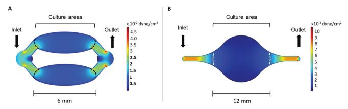
Fig. 3 COMSOL simulations of the wall shear stress in the (A) Ti-PDMS-chip and (B) Ti-glass-chip, in which the areas marked by the dashed lines indicate the border of the area designed for cell culture. The shear stress values marked in bold in the legend indicate the wall shear stress levels relevant to the cell culture areas
