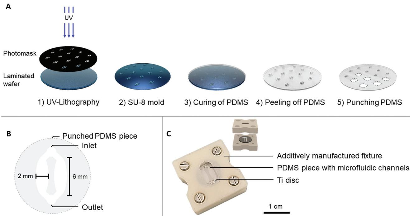
**Fig. 1** (A) Schematic of the process used to fabricate PDMS microfluidic channels for the Ti-PDMS-chip. (B) Schematic of one punched PDMS piece containing the two microfluidic channels. (C) Photograph of an assembled Ti-PDMS-chip and schematic of the opened chip to the side.
