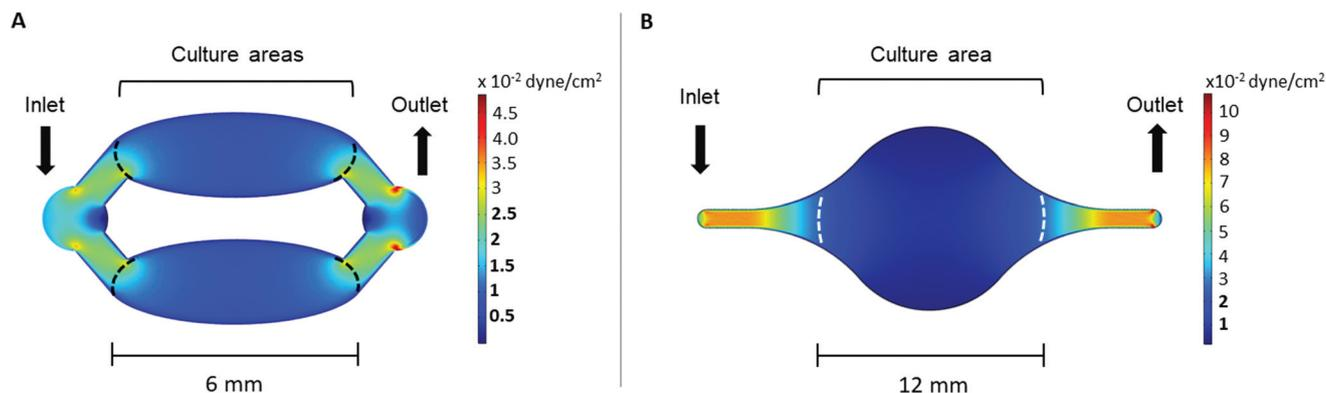
**Fig. 3** COMSOL simulations of the wall shear stress in the (A) Ti-PDMS-chip and (B) Ti-glass-chip, in which the areas marked by the dashed lines indicate the border of the area designed for cell culture. The shear stress values marked in bold in the legend indicate the wall shear stress levels relevant to the cell culture areas.
