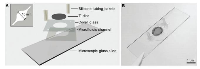
Fig. 2 (A) Schematic of the different layers constituting the Ti-glass-chip and (B) a top-view photograph of the completed device.
