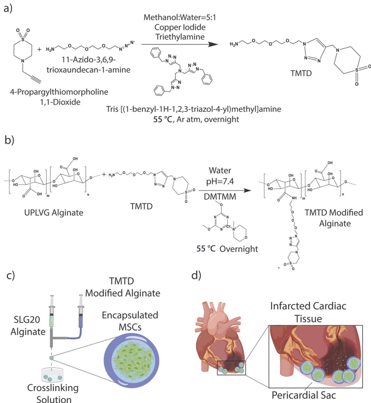
**Fig. 1** (a) Chemical schematic of TMTD small molecule synthesis and (b) TMTD small molecule modified alginate. (c) Schematic of electrostatic spraying mechanism used for encapsulation of MSCs into core shell capsules and (d) application of the platform in an acute myocardial infarct model.
