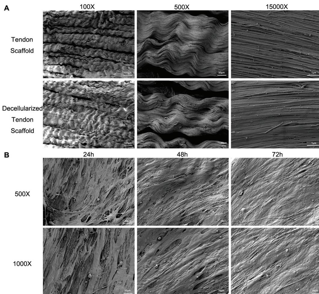
**Fig. 5** Scanning electron microscopy (SEM) of the scaffold and cell adhesion. Representative SEM images of (A) the scaffold without cells seeded, scale bar = 100 µm in 100x, 20 µm in 200x, 1 µm in 15 000x; and (B) the scaffold with cells seeded, scale bar = 10 µm.
