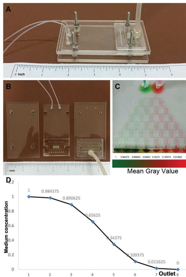
**Fig. 2** Manufacture and characterization of the microfluidic chip. (A) The integral structure of the microfluidic chip; (B) the three layers of the microfluidic chip; (C) the tree-like flow pattern in the microfluidic chip for the generation of a concentration gradient, and illustration with two dyes with a red and a green color; and (D) the medium concentration gradient created in the culture chamber.
