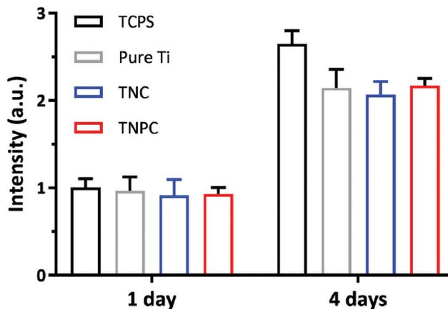
Fig. 5 *In vitro* cytotoxicity study of the pure Ti, TNC and TNPC with murine MC3T3-E1 osteoblastic cells determined by AlamarBlue assay at 1 and 4 days (error bars represent mean  $\pm$  standard deviation for  $n = 5$ ). MC3T3-E1 cell growth was unaffected by incubation with the pure Ti, TNC and TNPC for up to 4 days. No significant difference ( $p > 0.05$ ) in the viability of osteoblastic cells in contact with the TCPS (control group), pure Ti, TNC and TNPC.
