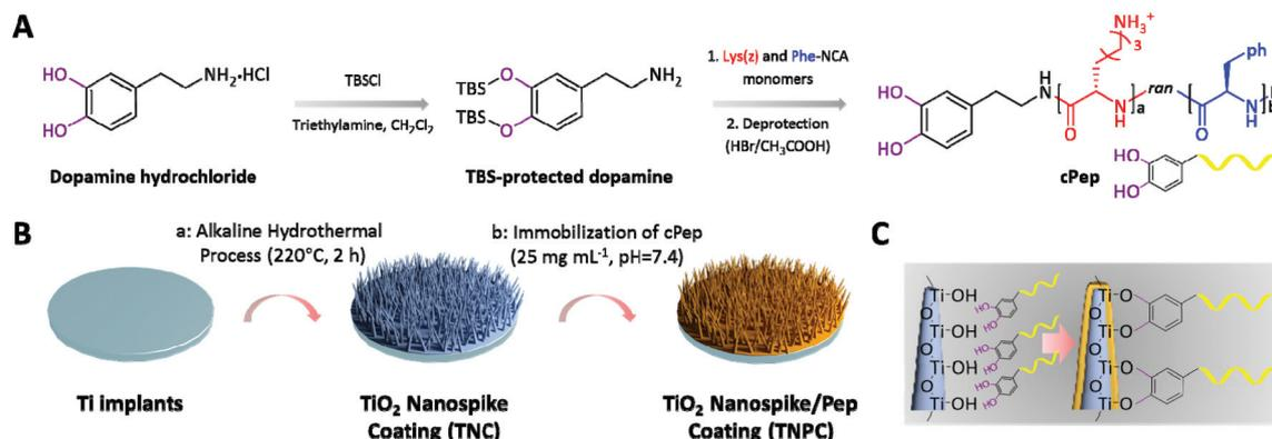
**Fig. 1** Illustration of the fabrication process of the TNPC. (A) The synthesis of antibacterial cPep. (B) The preparation of TNPC: (a) fabrication of TNC by an alkaline hydrothermal process; (b) immobilization of cPep onto TNC. (C) Coordinative interactions between catechol groups and TiO<sub>2</sub> nanospikes.
