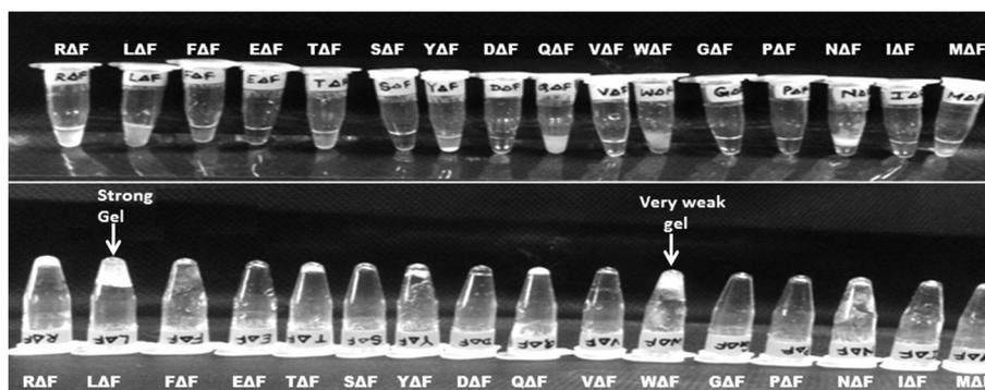
**Fig. 10** Tube inversion test showing the self-assembly of a set of modified dipeptides,  $X\Delta\text{Phe}$ , into a hydrogel. A dipeptide  $\text{Leu}\Delta\text{Phe}$ , instantaneously self-assembled into a self-supporting hydrogel.<sup>80</sup>
