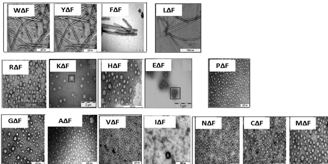
Fig. 7 TEM images showing the self-assembly of dipeptides containing a conformation-restricted residue,  $\alpha,\beta$ -dehydrophenylalanine at their C-terminal. Formation of self-assembled nanostructures by modified dipeptides (X $\Delta$ Phe) depending on their X-residue.
