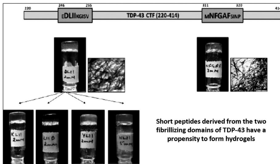
**Fig. 4** Hydrogel formation by short fragments derived from TDP-43 CFT (246–255) and TDP-43 CFT (311–320). Tube inversion test showing the formation of self-supportive hydrogels and their respective TEM images showing the presence of dense fibrillar mesh. Reprinted with permission from "A. Saini and V. S. Chauhan, Self-assembling properties of peptides derived from TDP-43 C-terminal fragment, *Langmuir*, 2014, 30(13), 3845–3856". Copyright (2014). American Chemical Society.
