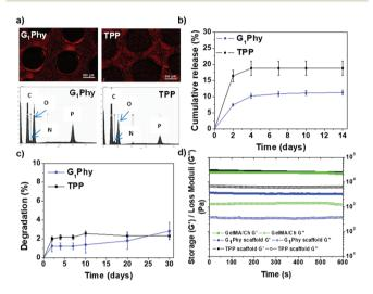
Fig. 5 (a) EDAX map distribution of P in G<sub>1</sub>Phy and TPP scaffolds, accompanied by EDAX spectra; (b) cumulative release crosslinker profiles for G<sub>1</sub>Phy and TPP scaffolds incubated in Tris-HCl buffer at pH 7.4 and 37 °C until 14 days; (c) degradation (%) for crosslinked scaffolds incubated in PBS at pH 7.4 and 37 °C until 30 days; (d) storage and loss moduli for UV-crosslinked GelMA/Ch gel and G<sub>1</sub>Phy and TPP scaffolds.
