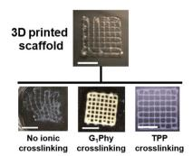
Fig. 3 Visual examination and structural integrity changes that a photochemically 3D printed scaffold (four layers) immediately experienced after immersion in distilled water containing or not the  $G_1$ Phy or TPP. Scale bar is 0.5 cm.
