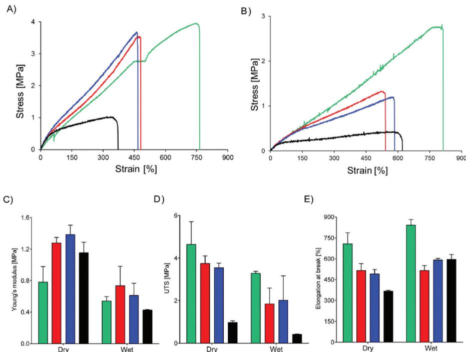
**Fig. 5** Mechanical properties of core-shell meshes in dry and wet conditions. Core polymer is UPy-PC (green), shell polymers are UPy-PEG<sub>600</sub> (red), UPy-PEG<sub>1000</sub> (blue), UPy-PEG<sub>1500</sub> (black). Representative stress-strain curves from uniaxial tensile test performed on meshes in the dry state (A) or swollen in water (B). Young's modulus (C), ultimate tensile strength (UTS) (D) and elongation at break (E) calculated from the stress-strain curves.
