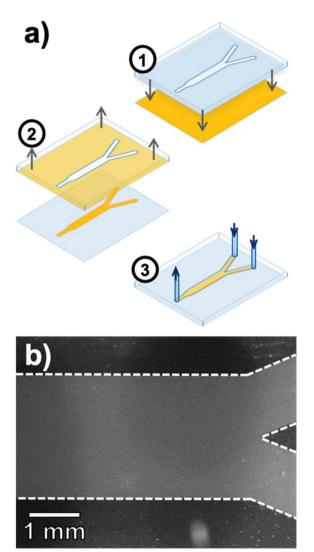
Fig. 13 (a) Fabrication steps for the pH-sensitive microfluidic Y-channel including (1) contact of the plasma-activated PDMS stamp with the Ag@ (FL) coated glass coverslip, (2) removal of the nanoparticle-bound stamp and (3) deposition of the PDMS microfluidic channel on the patterned glass surface. (b) Fluorescence image of the pH-sensitive channel after the stamping process. Adapted from ref. 123 with permission from the Royal Society of Chemistry, Copyright 2016.
