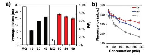
Fig. 9 (a) Fluorescence lifetime (left) and relative intensities  $(F/F_0, right)$  of MQ and In@(RB)@(FL)@MQ architectures with different silica thicknesses (in nanometres) in a 50 mM KCl solution in water (pH 6.4; N = 3). (b) Calibration curves of In@(RB)@(FL)@MQ (spacer thickness: 20 nm) with different halides (Cl⁻, Br⁻, l⁻) in aqueous solution (0.1 M phosphate buffer, pH 7.2; N = 3). Reproduced from ref. 103 with permission from the Royal Society of Chemistry, Copyright 2017.
