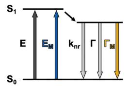
Fig. 1 Jablonski diagram for (a) a fluorophore excited in free-space conditions and (b) modified pathways in the vicinity of a plasmonic nanoparticle. E: excitation,  $k_{nr}$ : cumulative non-radiative decay rate,  $\Gamma$ : radiative decay rate. The M subscript represents metal-enhanced routes.
