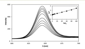
**Fig. 3** Emission spectra of 3D printed PtTFPP/SiO<sub>2</sub>/PLA indicator dot upon exposure to (from top to bottom): 0, 1, 3, 5, 10, 20, 40, 60, 80, 100% O<sub>2</sub>. Inset is a Stern–Volmer plot of the intensity data at 645 nm, illustrated in the main diagram, which a  $K_{\rm sv}$  value of (0.0142  $\pm$  0.0003) %O<sub>2</sub><sup>-1</sup> and a PO<sub>2</sub>(S = 1/2) value of 70.4%O<sub>2</sub>.
