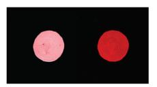
Fig. 1 Photographs of a 30  $\mu$ m thick 3D printed PtTFPP/SiO<sub>2</sub>/LDPE indicator dot with 1 cm diameter taken under daylight in air (left), and under UV light in an Ar atmosphere (right).
