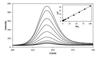
Fig. 2 Emission spectra of 3D printed PtTFPP/SiO<sub>2</sub>/LDPE indicator dot upon exposure to (from top to bottom): 0, 1, 3, 5, 10, 20, 40, 60, 80, 100% O2. Inset is a Stern-Volmer plot of the intensity data at 642 nm, illustrated in the main diagram, which a  $K_{\rm sv}$  value of (0.205  $\pm$  0.002) %  $O_2^{-1}$  and a  $PO_2(S = 1/2)$  value of 4.88% $O_2$ .
