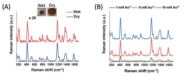
Fig. 4 (A) Comparison of the SERS spectra of 2  $\mu$ M MGITC under wet and dry conditions using 10 mM Au@Fe<sub>3</sub>O<sub>4</sub>@BCNCs. Inset pictures show before/after drying of 10  $\mu$ L of the droplet including the nanocomposites. (B) The SERS spectra of 2  $\mu$ M MGITC using the Au@Fe<sub>3</sub>O<sub>4</sub>@BCNCs with different Au coating condition (1, 5, and 10 mM Au<sup>3+</sup>). All spectra shown here are the average of 400 collected spectra.
