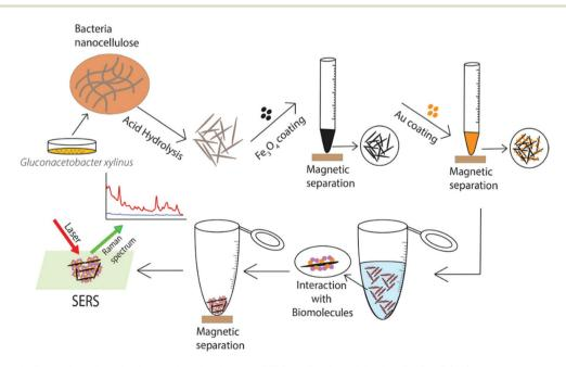
$\begin{tabular}{ll} Schematic illustration of synthesis, functionalization, and SERS application of the Au@Fe_3O_4@BCNCs. The supplies of the A$
