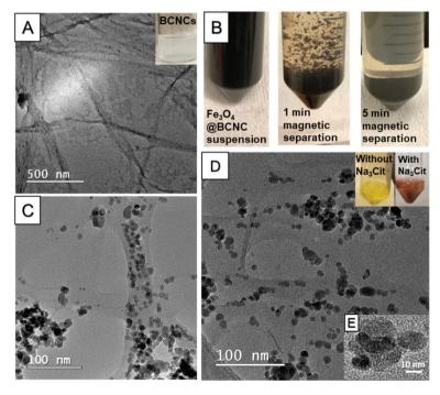
Fig. 1 (A) TEM image of as-synthesized BCNCs, (B) Fe<sub>3</sub>O<sub>4</sub> coated BCNCs in suspension and magnetically separated, (C) TEM image of Fe<sub>3</sub>O<sub>4</sub>@BCNCs, (D) TEM image of Au@Fe<sub>3</sub>O<sub>4</sub>@BCNCs and (E) Au and Fe<sub>3</sub>O<sub>4</sub> nanoparticles.
