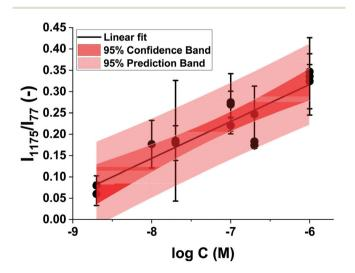
Fig. 6 The comprehensive plot of the normalized Raman peak of 1175 cm $^{-1}$  vs. the logarithm of the concentrations of MGITC using 1, 5, and 10 mM Au@Fe $_3$ O $_4$ @BCNCs. The black solid line shows the best-fit linear curve. Dark and light red-colored regions show statistical 95% confidence and prediction bands, respectively.  $R^2=0.79$ , Linear fit:  $I_{1175}/I_{77}=0.837+0.087\log C$ .
