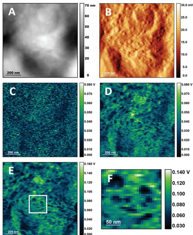
**Fig. 4** PTIR images of the cellular surface of buccal cells with resonant-mode excitation. A. AFM height image of a cell surface. B. AFM deflection image of the same region as in A. C–E. PTIR images of the same region as in A using 1654  $\text{cm}^{-1}$  excitation and 65 kHz, 312 kHz and 821 kHz pulsing frequency respectively. F. Detail of E showing surface structures. No resonance tracking was implemented for these images.
