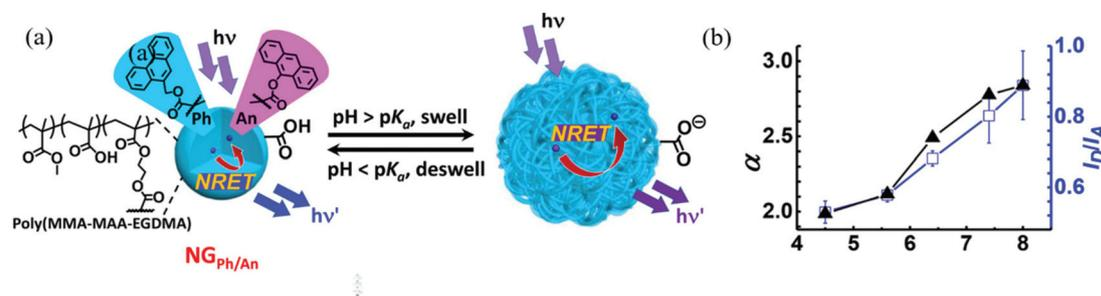
Fig. 3 (a) Schematic depicting the sensing mechanism of pH-responsive nanogel probes (NGPh/An). (b) Variation of the average linear swelling ratio ( $\alpha$ ) and  $I_{Ph}/I_{An}$  with pH for DX NG(NGPh/An). Reprinted (adapted) with permission from ref. 67. Copyright (2017) American Chemical Society.
