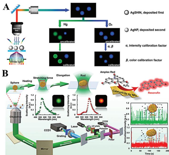
**Fig. 6** (A) Schematic of the enlarged color-coded dark-field image of amalgamation using Ag NPs as the reference. Reprinted with permission from ref. 81. Copyright 2019, American Chemical Society. (B) Schematic diagram of the procedures for laser-controlled shape modulation and single-molecule catalysis from gold nanostructures with different morphologies. Reprinted with permission from ref. 88. Copyright 2019, Royal Society of Chemistry.
