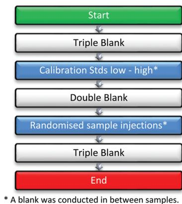
Fig. 2 Sequence of the samples during the analyses.
