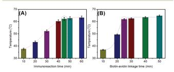
Fig. 3 Dependence of temperature on (A) immunoreaction time and (B) the biotin-avidin linkage time of the photothermal immunoassay (10 ng mL<sup>-1</sup> NSE used in these cases).
