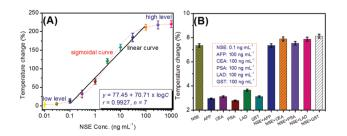
Fig. 4 (A) Calibration plots of the photothermal immunoassay towards NSE levels by using PBNP-liposomes as the signal-generation tags at 1.5 V under 808 nm NIR-light irradiation and (B) the specificity of photothermal immunoassay against NSE, AFP, CEA, PSA, LAD, and GST.
