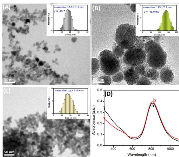
**Fig. 1** Typical TEM images of (A) Prussian blue nanoparticles (inset: DLS data including size distribution and zeta potential), (B) PBNP-liposomes (inset: DLS data including size distribution and zeta potential), and (C) PBNP-liposomes (inset: DLS data); (D) Vis-NIR spectra of (a) Prussian blue nanoparticles and (b) PBNP-liposomes + Tween 20.
