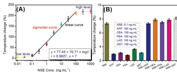
**Fig. 4** (A) Calibration plots of the photothermal immunoassay towards NSE levels by using PBNP-liposomes as the signal-generation tags at 1000 V under 808 nm NIR-light irradiation and (B) the specificity of photothermal immunoassay against NSE, AFP, CEA, PSA, LAD, and GST.
