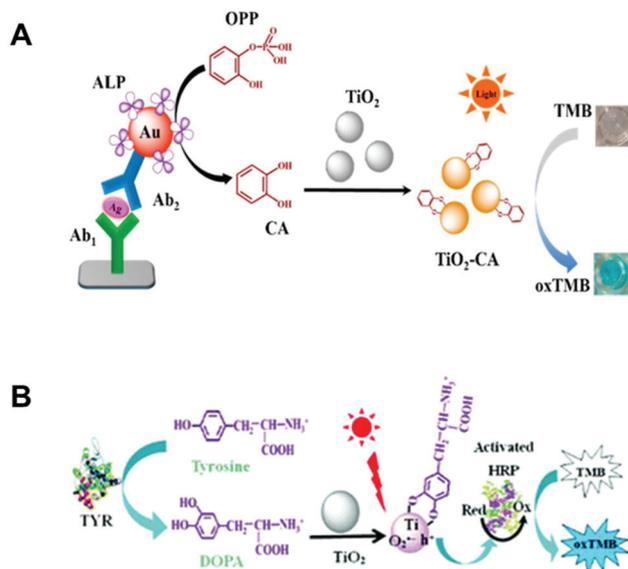
Fig. 7 (A) Proposed immunodetection process for mouse IgG by coupling the *in situ*-generated photo-responsive nanozyme of CA- $TiO_2$ . (B) Schematic illustration of the colorimetric sensing mechanism for TYR based on the photoactive sensor. (A) Reproduced from ref. 79 with permission from the American Chemical Society, copyright 2015. (B) Reproduced from ref. 80 with permission from the Royal Society of Chemistry, copyright 2017.
