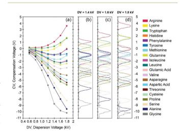
Fig. 1 Differential ion mobility data for 20 protonated AAs recorded at different dispersion voltage (DV) using N2 as carrier gas. (a) DMS dispersion plots, or evolution of CV as a function of DV; DMS spectra for each individual AA at DV = 1.4, 1.6, 1.8 kV are given in panels (b), (c), and (d), respectively. A CV value of 1 V corresponds to an electric field of 1.43 kV  $m^{-1}$  or  $\sim$ 0.07 Td. To facilitate visualization, each DMS peak is individually normalized.
