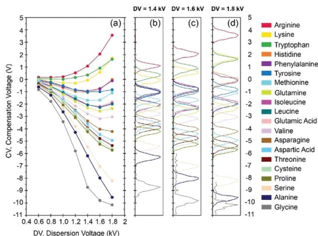
**Fig. 1** Differential ion mobility data for 20 protonated AAs recorded at different dispersion voltage (DV) using  $\text{N}_2$  as carrier gas. (a) DMS dispersion plots, or evolution of CV as a function of DV; DMS spectra for each individual AA at DV = 1.4, 1.6, 1.8 kV are given in panels (b), (c), and (d), respectively. A CV value of 1 V corresponds to an electric field of 1.43  $\text{kV m}^{-1}$  or  $\sim 0.07$  Td. To facilitate visualization, each DMS peak is individually normalized.
