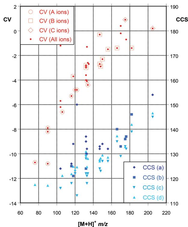
Fig. 2 CV and CCS as a function of  $m/z$  for a selected set of AAs and related species (see list in Table S4†). CV values (in V), 1 V corresponding to an electric field of  $1.43 \text{ kV m}^{-1}$  or  $\sim 0.07 \text{ Td}$ . CCS (in  $\text{\AA}^2$ ) are taken from (a) ref. 38, (b) ref. 33, (c) ref. 17, and (d) ref. 51.
