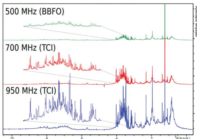
**Fig. 5** Demonstration of magnetic field strength and probe specificity on spectral resolution of bovine serum recorded with the same parameter set on three spectrometers working at 500, 700, and 950 MHz proton frequencies at 25 °C. Figure reproduced from ref. 5 under Creative Commons Attribution 4.0 International License (<http://creativecommons.org/licenses/by/4.0/>).
