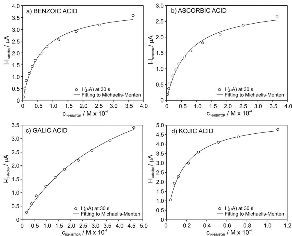
Fig. 5 Plot of the absolute current change for increasing concentrations of the inhibitors in the presence of  $4 \times 10^{-4}$  M catechol concentration in PB: (a) benzoic acid, (b) ascorbic acid, (c) gallic acid, and (d) kojic acid.
