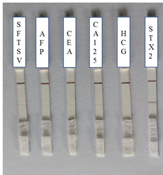
Fig. 4 Specificity test of Au NP based LFITS (from left to right: SFTSV, AFP, CEA, CA125, HCG and STX2, the concentrations of antigens were  $1 \mu\text{g mL}^{-1}$ ).
