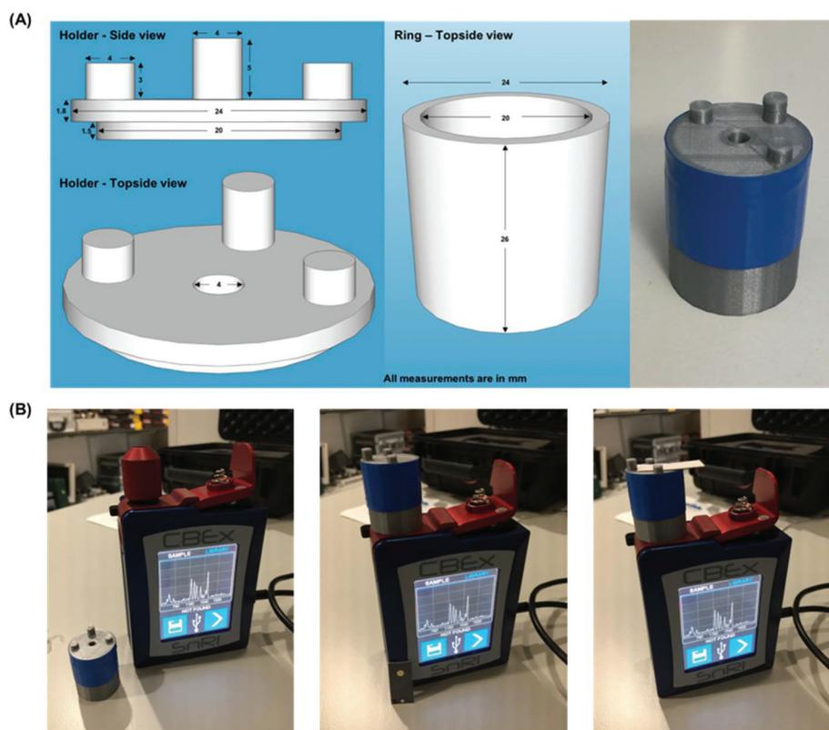
Fig. 2 (A) shows the design and dimensions of the Raman aperture adaptor used for the analysis of the capture layer contained within the 3-D paper device. The adaptor was appropriately scaled to ensure that readouts were made at the optimal distance and center of the spot (B) Images display how the adaptor fits over the point and shoot lens and how the capture layer is mounted to enable SERS analysis.
