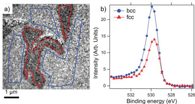
Fig. 6 (a) XPEEM image at the oxygen 1s core level after exposing the phase-separated alloy surface to 8.4 L O<sub>2</sub>. The dark (bright) regions, highlighted by the red (blue) contours, correspond to the fcc (bcc) areas. (b) The XPS spectra from the bcc and fcc regions, which are marked on the XPEEM image.
