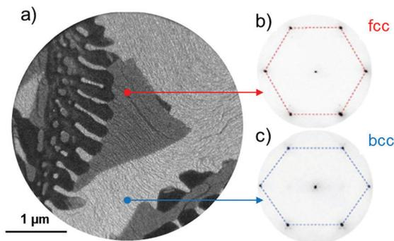
Fig. 1 (a) LEEM image of the phase separated FeNi film. Electron energy is 21 eV. The  $\mu$ -LEED patterns from (b) gray (fcc) and (c) bright (bcc) regions are acquired at 65 eV. The finger-like dark regions in the LEEM image correspond to dewetting.
