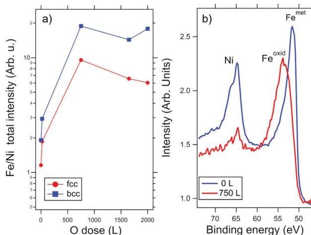
Fig. 2 (a) Evolution of the Fe 3p and Ni 3p core-level intensity ratio as a function of  $\text{O}_2$  exposure. (b) Comparison of the XPS spectra at the two core levels acquired upon 0 L and 750 L oxygen exposure. Photon energy is 250 eV.
