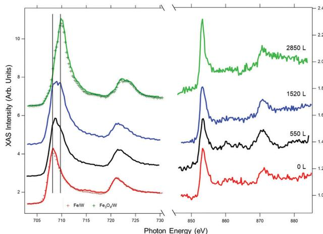
Fig. 3 Integrated XAS measurements at the Fe  $L_{2,3}$ - and Ni  $L_{2,3}$  edges for a  $\text{Fe}_{0.7}\text{Ni}_{0.3}$  thin film upon increasing  $\text{O}_2$  exposure. The reference Fe L-edge spectrum of metallic Fe/W and  $\text{Fe}_3\text{O}_4/\text{W}$  samples are superimposed to the first and last spectra.
