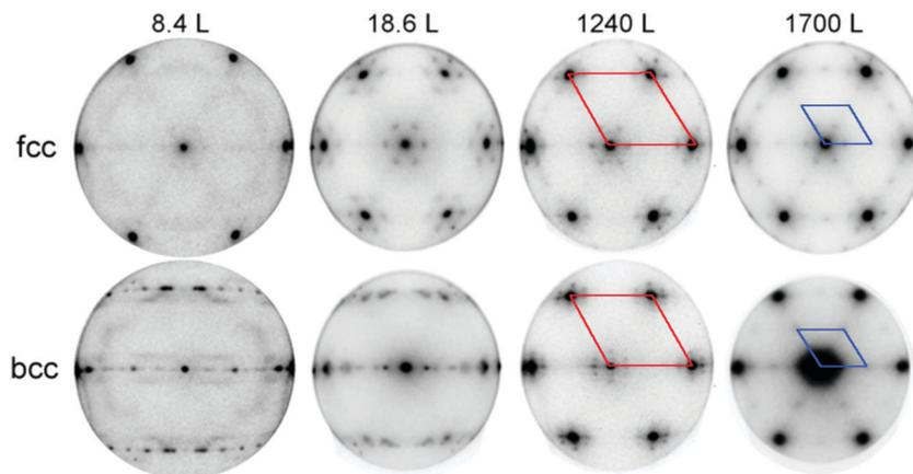
Fig. 5  $\mu$ -LEED patterns as a function of oxygen dose for the fcc (top row) and bcc (bottom row) phases present in the phase-separated alloy surface. The electron energy is 45 eV. The unit cell for the FeO and Fe<sub>3</sub>O<sub>4</sub> phases is indicated in the image (red and blue lines, respectively); the substrate [110] direction is along the horizontal axis.
