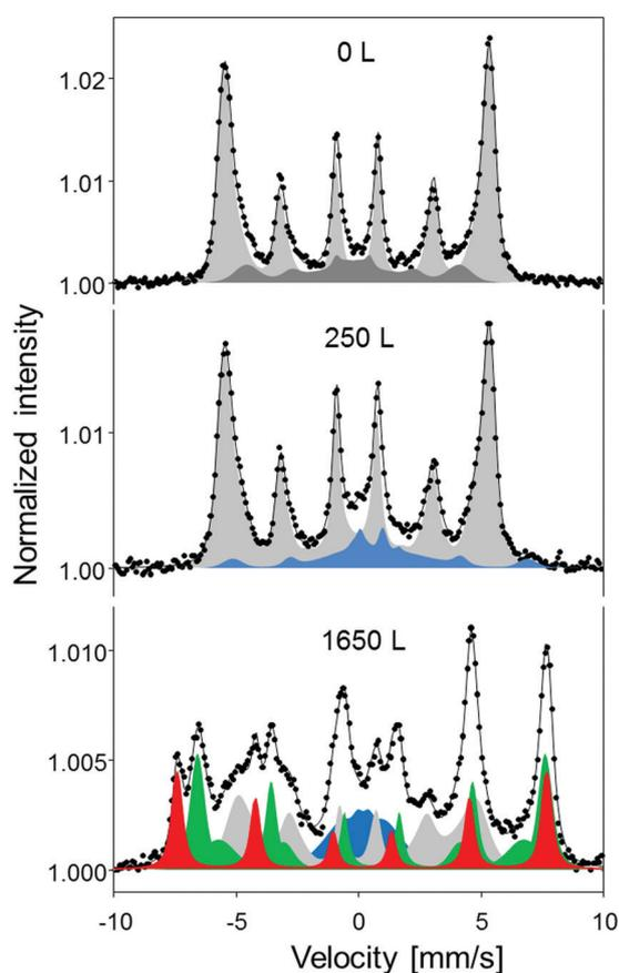
**Fig. 4** CEMS spectra of the Fe<sub>0.7</sub>Ni<sub>0.3</sub> film are shown for varying oxygen dose. The measurement averages over both fcc and bcc phases of the phase-separated alloy film. The spectral components are color-coded: light gray – metallic FeNi; red – the tetrahedral site in the spinel; green – the octahedral site in the spinel; and blue – non-specific oxide components. For the top spectrum of the pristine film the decomposition into bcc-FeNi (light gray) and fcc-FeNi is shown.
