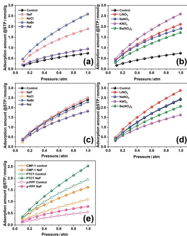
Fig. 5 CO<sub>2</sub> adsorption isotherm at 273 K of PTAPA (a and b), PAPA (c and d), and CMP-1, PTCT & *p*-PPF (e) before and after tuning by BXJ salts.
