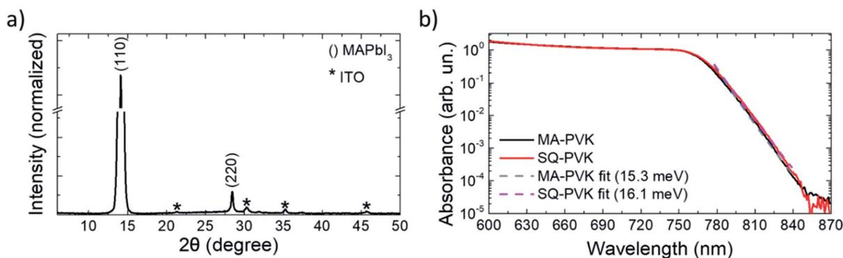
Fig. 3 (a) XRD pattern of the MA-treated perovskite film. The CH<sub>3</sub>NH<sub>3</sub>PbI<sub>3</sub> related peaks are indexed in parentheses, whereas the substrate related peaks are marked with a \* (Fig. S10†). (b) PDS spectra of solvent quenched MAPbI<sub>3</sub> and of MA-PVK. Fits to the experimental data are also shown in the figure.
