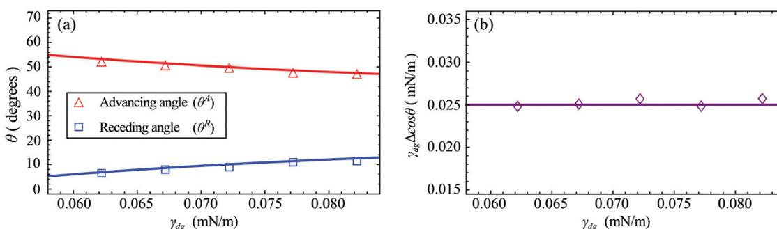
Fig. 4 (a) The effect of  $\gamma_{dg}$  on  $\theta^A$  and  $\theta^R$ . The red and blue lines are the theoretical predictions for  $\theta^A$  and  $\theta^R$  as given in eqn (18) and (19) respectively. (b) The pinning force per unit length for a droplet on LIS is independent of  $\gamma_{dg}$ .
