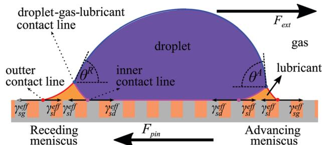
Fig. 1 Droplet on LIS under influence of an external force  $F_{\text{ext}}$ . The resisting force due to contact line pinning,  $F_{\text{pin}}$ , is pointing in the opposite direction. We have also shown the surface tension forces acting on the inner and outer contact lines.
