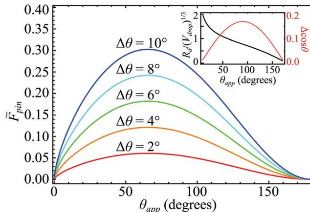
Fig. 6 Visualisation of the effects of CAH and the droplet shape on the pinning force. The inset shows the non-dimensionalised droplet base radius  $R_d/\sqrt[3]{V_{\text{drop}}}$  and  $\Delta \cos \theta$  against  $\theta_{\text{app}}$ .
