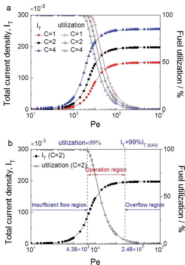
Fig. 15 (a) Dependence of dimensionless total current density  $I_T$  and fuel utilization with dimensionless parameter  $Pe$  at different dimensionless concentration  $C$  and (b) three different flow regimes distinguished ( $V_{\text{cell}} = 0.6 \text{ V}$ ). Reproduced with permission from Elsevier.<sup>295</sup>
