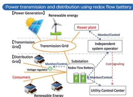
Fig. 17 One of the largest RFB systems (2 MW/8 MW h) developed by Sumitomo and NEDO for systems integration in the US. Reproduced with permission from Green Car Congress, SEI.<sup>341</sup>
