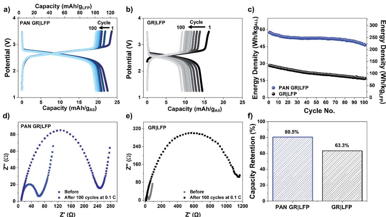
Fig. 4 Charge discharge curves of every 10<sup>th</sup> cycle of galvanostatic cycling at 0.1 C for (a) PAN GR|LFP and (b) GR|LFP full-cells, (c) energy density vs. cycle number with respect to total mass (left y-axis) and LFP active material (right y-axis), electrochemical impedance spectroscopy spectra of (d) PAN GR|LFP and (e) GR|LFP full-cells before and after 100 cycles at 0.1 C, and (f) capacity retention over 100 cycles at 0.1 C.
