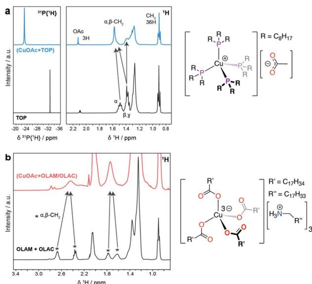
Fig. 4 Characterization of the precursor solutions. (a) <sup>31</sup>P{<sup>1</sup>H} NMR spectra and <sup>1</sup>H NMR spectra of the Cu complex formed by a combination of CuOAc and TOP. (b) <sup>1</sup>H NMR spectra of the Cu complex formed by a combination of CuOAc, OLAM and OLAC. The proposed molecular structures of the Cu complexes in each mixture are shown on the right of the corresponding spectra.
