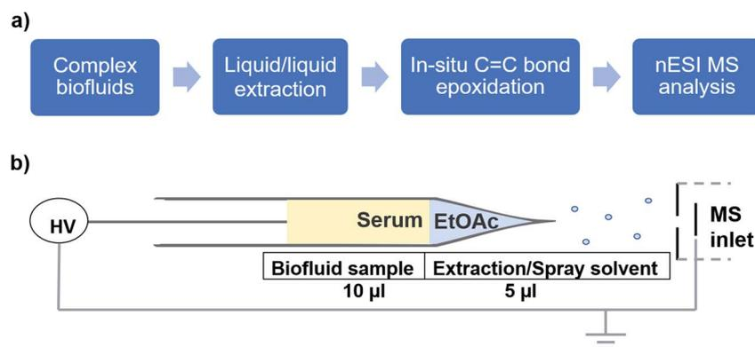
Fig. 4 (a) Sequence of the experimental approach for complex biofluid analysis involving in-capillary extraction, *in situ* oxide creation and epoxidation, and real-time analysis by nESI MS. (b) Schematic illustration of the platform for in-capillary liquid/liquid extraction of FFAs from serum using ethyl acetate and subsequent MS analysis with nESI using Ir where *in situ* fatty acid epoxidation occurs.
