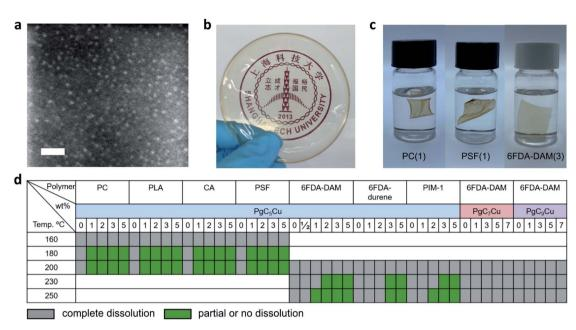
Fig. 1 Qualitative dissolution analyses for various  $PgC_nCu$ -polymer composite membranes. (a) STEM image of  $PgC_5Cu$ , scale bar 10 nm. (b) A photograph of a 6FDA-DAM(2) membrane. (c) Photographs of PC(1), PSF(1) and 6FDA-DAM(3) immersed in DCM. (d) Dissolution table of various neat polymers and their composite membranes with  $PgC_nCu$ .
